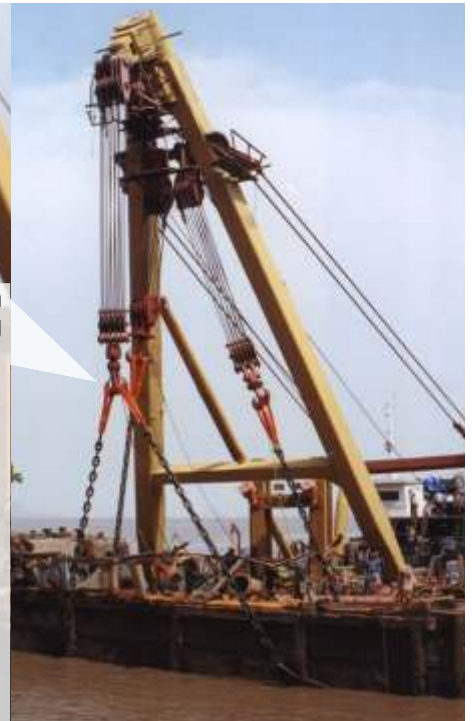
The sunken 280 ton Indira Gate being lifted using our Zebra Round Slings.
