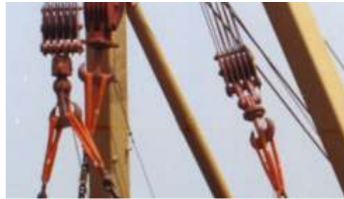
The sunken 280 ton Indira Gate being lifted using our Zebra Round Slings.
